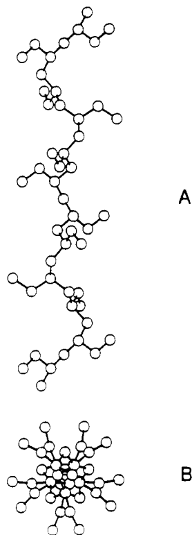
Figure 12. Side view (A) and a projection along the chain axis (B) of the model suggested for the chain conformation of form II of s-PB.
